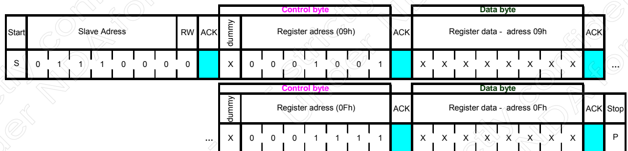
Figure 15: I 2 C multiple write protocol
